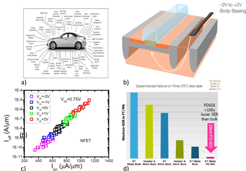
Figure 1: a) electronic parts for typical vehicle [source: Clemson University Vehicular Electronics Lab]; b) FD-SOI device with Back Bias [Globalfoundries, "FD-SOI Technology Innovations Extend Moore's Law" white paper, September 2015, <http://globalfoundries.com/>]; c) Ion
